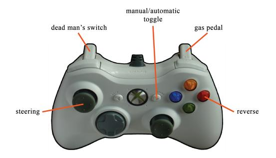
Figure 7.2: Control scheme for an Xbox 360 controller, mapping buttons to control actions.
