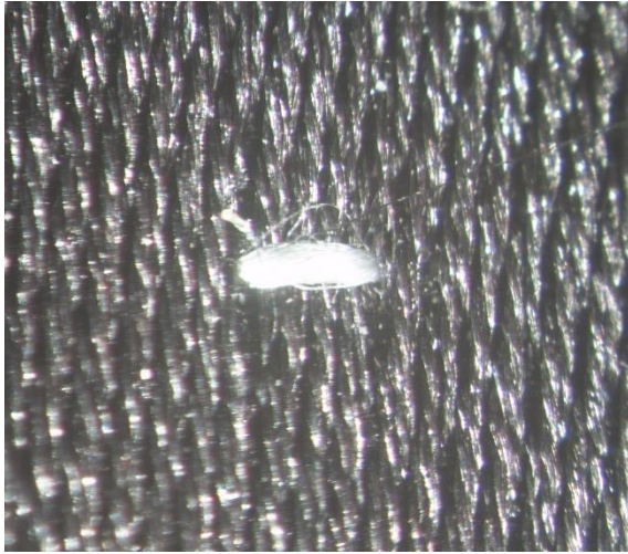
Figure 24. Stereomicroscope photograph of specimen AVSF at the centre bottom stitch holding the support fabric, before the fixed-load test. Photo: Marie Schön
