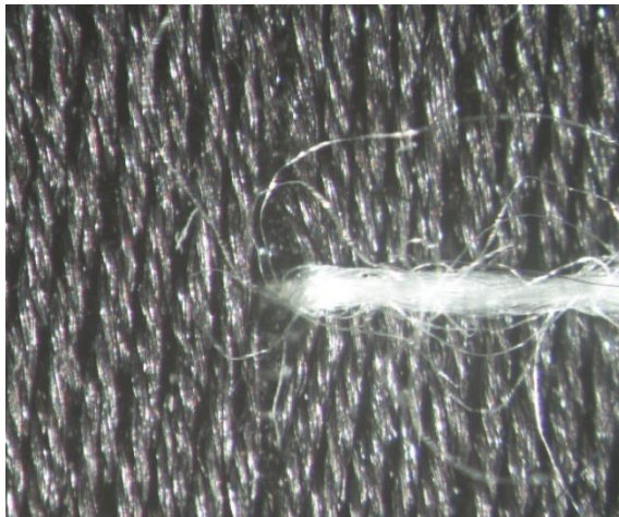
Figure 20. Stereomicroscope photograph of specimen AVL2 I at the left end of the top laid stitch, before the fixed-load test. Distortion at the end of the stitch. Photo: Marie Schön
