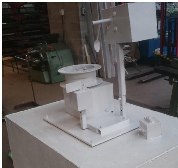
It's constructed of three different electrical motors. One big motor with the force of 0,5 horse powers, which is strong. On to this motor i mounted a plastic cylinder which is a bit off center, making it oscilate and vibrate a lot. I had to fixate it to six pallets so that it wouldn't shake to pieces. Together with this motor there are two more, one smaller just next to the big one which spins closely to it with a small tool to help spread the paint in to finer particles.
