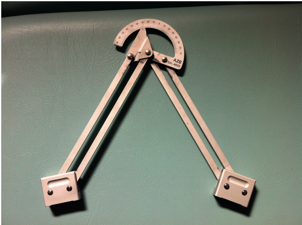
Figure 27: The Debrunner Kyphometer.
