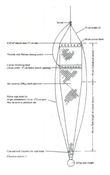
Fig.2. The type of net proposed by Working Party no.2 inside UNESCO for taking smaller mesoplankton (Tranter, 1968).
