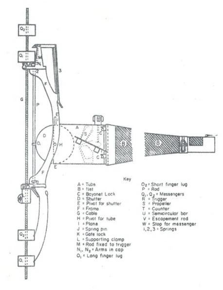
Fig.6. The Clarke-Bumpus plankton sampler (from Edmondson & Winberg, 1971).
