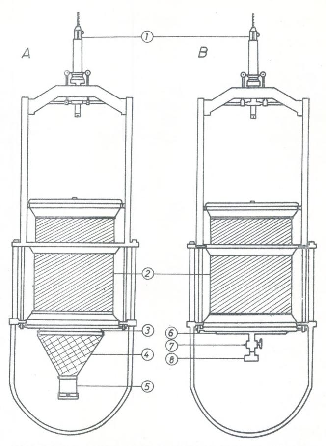
Fig.1. A plankton sampler with a capacity of 23 litres. A) The sampler is modified for taking zooplankton samples. B)The sampler is modified for taking phytoplankton and water samples (Ackefors, 1971a). 0 10 20 30 40 50 60 cm
