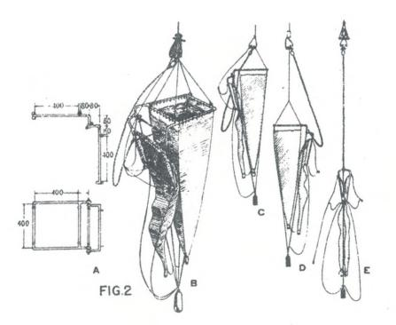
Fig.5. The Motoda net for vertical hauls ( Motoda, 1963).
