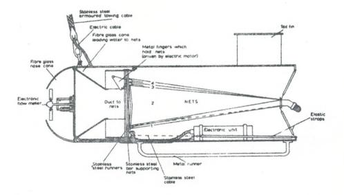
Fig.12. The net-changing device for use with the Lowestoft multipurpose sampler (Harding et al., 1971).
