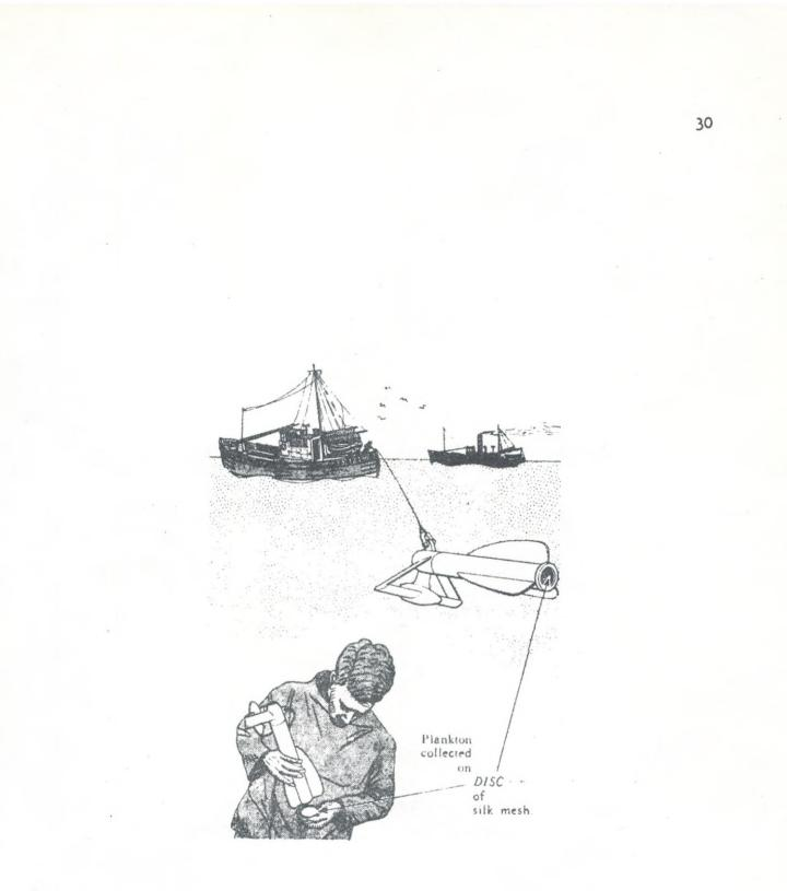
Fig.9. The Hardy Plankton Indicator, as used to sample plankton by fishing vessels working on the herring grounds (Fraser, 1962).
