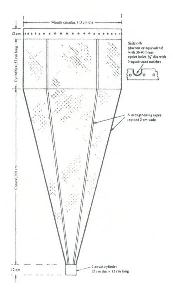
Fig.13. The simple unencased net ' the interim net ' proposed by the Working Party no.3. inside UNESCO for taking larger mesozooplankton (Tranter ,1968).
