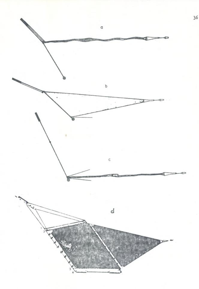
Fig.15. The operation of the rectangular opening-closing trawl; a) the net is payed out to the fishing depth b) the open position c) after closure while it is hauled to the surface d) the rectangular opening--closing trawl in the open, fishing position ( Clarke .1969).
