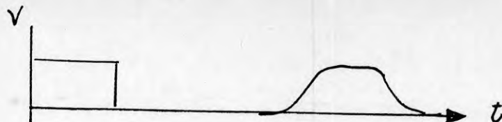
Figur 3.11:4. Dispersion i fiber
