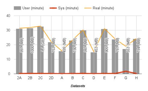
Figure 3.2. CPU time and elapsed time spent for pre-processing and quality control of dataset using SolexaQA software. Real is total elapsed time including I/O; User is CPU time spent in the user-mode code and Sys is CPU time spent in the kernel. Label on the bars shows the size of datasets.
