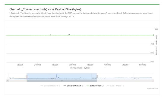
Figure 5.5: Chart of t\_Connect against payload size.
