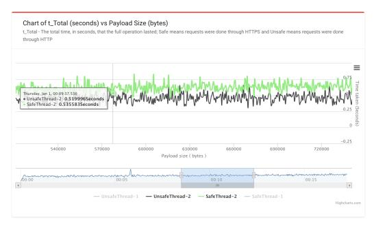
Figure 5.10: Chart of t\_Total against payload size.
