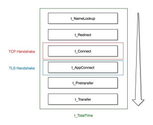
Figure 4.6: Quantities measured in this test in order of appearance in HTTP call.
