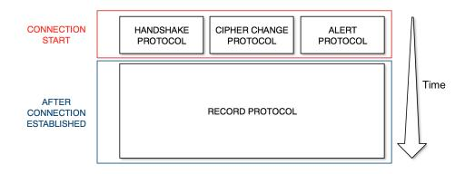
Figure 2.1: TLS Protocol Stack with respect to time each part is being used.
