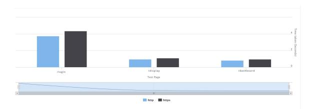
Figure 5.1: Chart of time taken for web pages to load when HTTP is used against when HTTPS is used.
