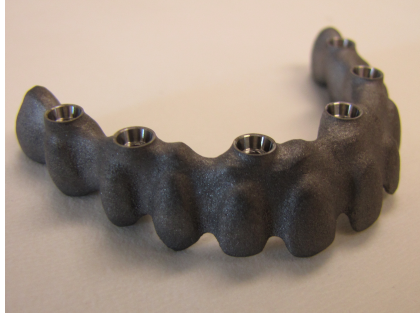
Figure 9. AM CoCr framework before ceramic veneering.
