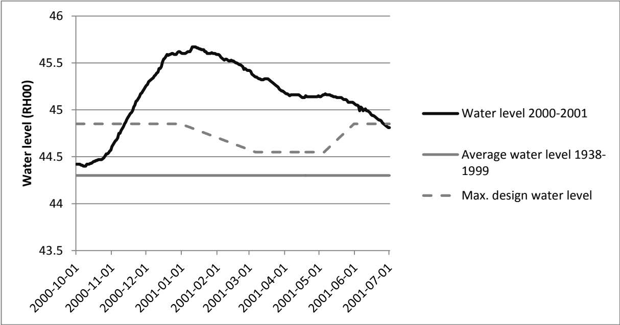
Figure 2: Time series of the water level in Vänern from October 2000 to June 2001.
