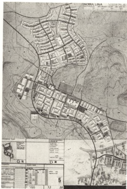
FIG. 2. Alternative housing area plan (1:2000) for Norra Lina, Södertälje, produced from a sketch model to the scale 1:1000.
