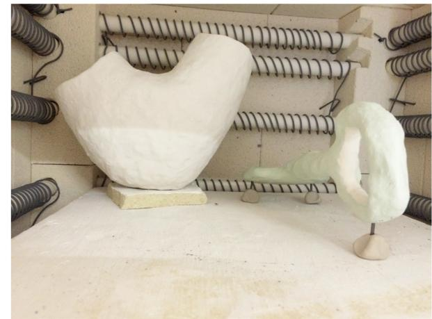
Packing the kiln with some of the objects I made. On these two pictures you can see some kiln-stands I made out of clay and a kanthal wire to avoid the sculptures from getting stuck onto the kiln shelves.
