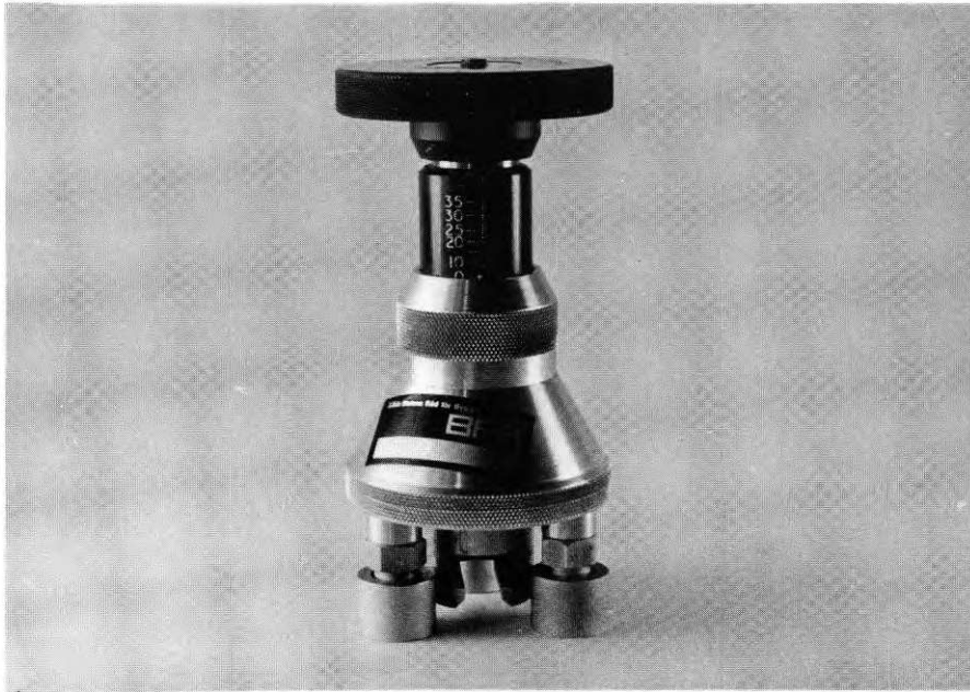
FIG.5. Mekanisk dragprovare typ "Elcometer Adhesion Tester". Mechanical tensile tester type "Elcometer Adhesion Tester".
