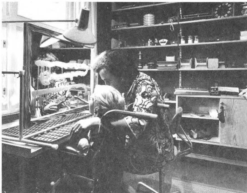
FIG. 1. Elocution and sensory function training in a room for individual teaching. Children with perception disability and lack of concentration are confused by looking at the objects on the shelves and the view from the window. The window should be of a clearstorey type and the open shelves replaced either by a cupboard or by some form of screen. (Foto by Bengt Carlén.)
