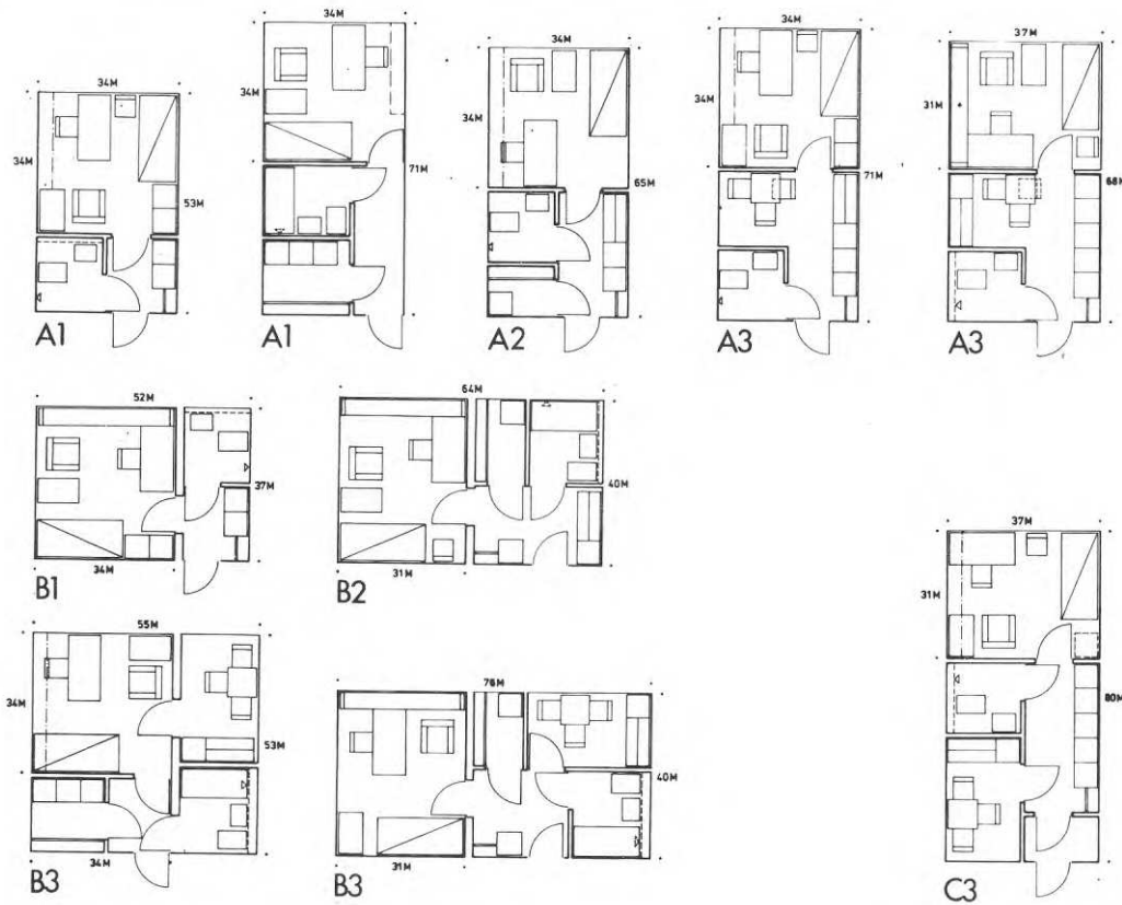
FIG. 3. Plans of flats. Scale 1:200. Each flat is coded according to series (A, B, C) and standard (1, 2, 3).
