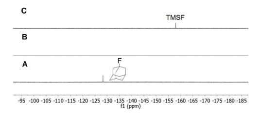
**Figure 4.** <sup>19</sup>F NMR spectra of **A**: 1-fluoroadamantane in CD<sub>2</sub>Cl<sub>2</sub>. **B**: No fluorine signal observable due to instantaneous and quantitative conversion of 1-fluoroadamantane to 1-iodoadamantane upon addition of YbI<sub>3</sub>(THF)<sub>3</sub> to **A**. **C**: Further addition of TMSI reveal instantaneous formation of TMSF.
