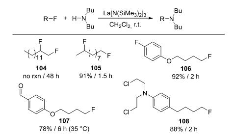
Scheme 29. The La[N(SiMe<sub>3</sub>)<sub>2</sub>]<sub>3</sub> mediated amination of functionalized alkyl fluorides.
