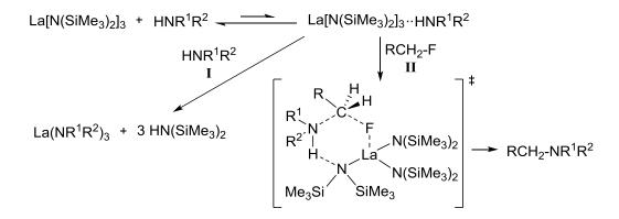
Scheme 30. Proposed mechanism for the La[N(SiMe<sub>3</sub>)<sub>2</sub>]<sub>3</sub> mediated amination of an alkyl fluoride.
