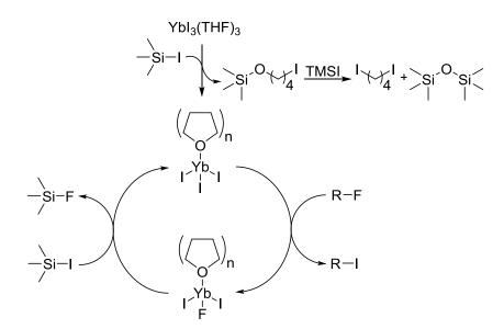
Scheme 23. Proposed catalytic cycle for the  $YbI_3(THF)_n$  catalyzed C–F bond substitution in presence of TMSI. n=0-3 THF ligands.
