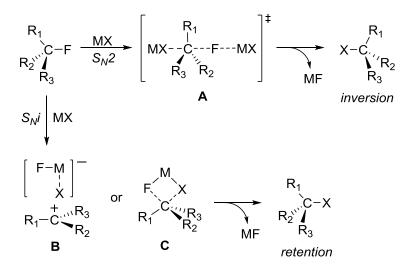
**Scheme 21.** Mechanistic proposal for the C–F bond activation mediated by YbI<sub>3</sub>(THF)<sub>3</sub>. MX= YbI<sub>3</sub>(THF)<sub>3</sub>. MF= YbI<sub>2</sub>F(THF)<sub>3</sub>.
