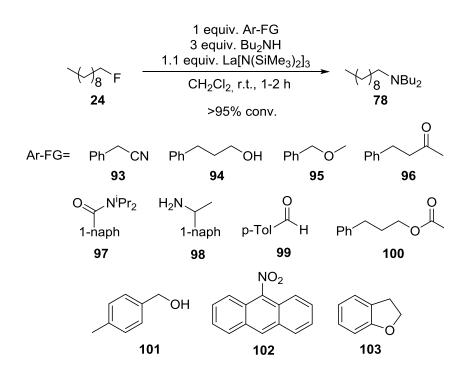
**Scheme 28.** A chemoselective study of the La[N(SiMe<sub>3</sub>)<sub>2</sub>]<sub>3</sub> assisted amination of 1-fluorodecane upon separate addition of various substrates containing common functional groups.
