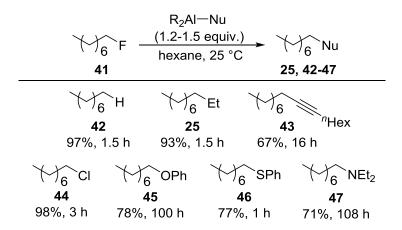
Scheme 14. Several examples on triorganoaluminium mediated functionalization of 1-fluorooctane.
