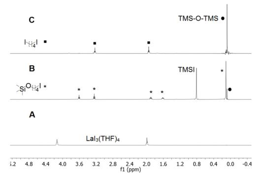
**Figure 5.** <sup>1</sup>H NMR spectra of **A**: THF signals from  $LaI_3$ (THF)<sub>4</sub> in CD<sub>2</sub>Cl<sub>2</sub>. **B**: Spectra obtained 5 min after addition of TMSI showing quantitative ring-opening of THF to yield (4-iodobutoxy)trimethylsilane. **C**: After additional 18 h only 1,4-diiodobutane and hexamethyldisiloxane is detected.
