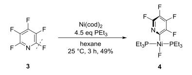
Scheme 4. Selective activation of pentafluoropyridine using stoichiometric amount of Ni(0).
