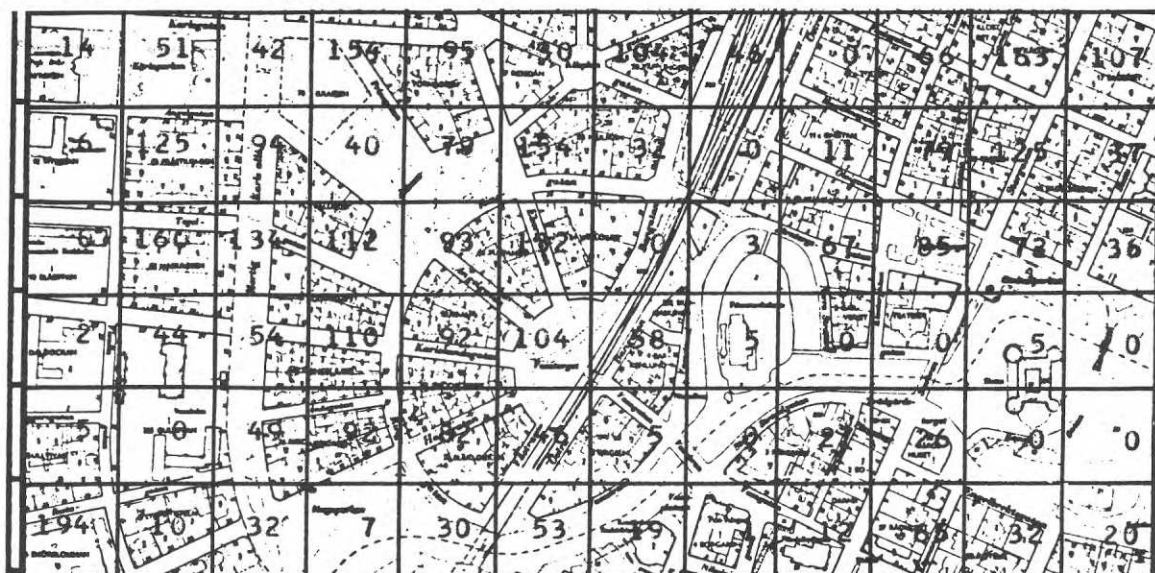
FIG. 3. Grid map from line printer superimposed on ordinary map, central areas of Örebro. Grid size 100x100 m 2 .
