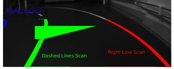
average frame is demonstrated in Figure 24. As low as 8% of the image traversed, much more efficient than looping through the whole image with OpenCV's find contours function.
