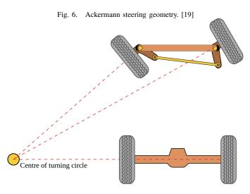
Only cars based on Ackermann steering, or variations of, are allowed to compete [Fig. 6]. Ackermann steering is the standard for commonly met automobiles.
