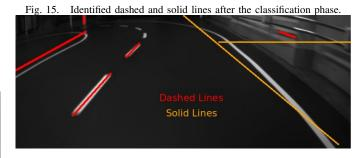
1) Classify Lines: The rectangles are approximated into lines according to their vertices and are then classified into solid or dashed lines. The classification is done by comparing the ratio between width and height of the rectangles or their length compared to the longest rectangle [Fig. 15]. Sometimes, solid lines may be miss-classified as dashed lines, this step of the algorithm is ran again during later phases to minimise this risk.
