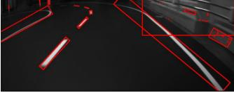
*3) Get Rectangles:* Each approximated contour is then transformed into an OpenCV Rotated Rectangle [Fig. 14]. This data structure helps us find out the angle each contour is rotated at.
