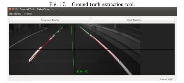
The ground truth data creator tool is able to load recordings and traverse them both forwards and backwards while displaying each frame in the main window. Its main purpose is to let us draw the lines that form the vanishing point in a visual and user friendly way [Fig. 17].
