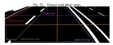
An overview of the extract road steps is shown in [Fig. 23] We use pointers to loop through and access the contents of a matrix. Looping through a matrix using a pointer is the fastest way, OpenCV's at() function is designed for random access [45]. The reach of the extract road algorithm of an
