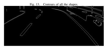
1) Find Contours: With the help of OpenCV, it is possible to get the contours of all the shapes in the frame [42] [Fig.
