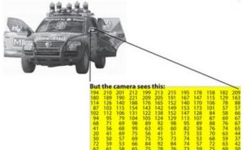
as a matrix of colours [Fig. 1, 2]. Each matrix element holding an array of integers describing the colour using a combination of colour channels, e.g. red, green and blue; cyan, magenta, yellow and black; shades of grey; black and white. An element, unit or item of an image matrix is often referred to as *pixel*.
