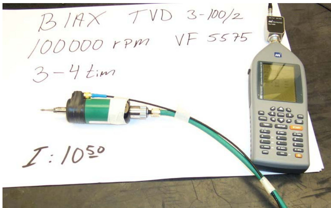
Figure 3: The accelerometer is taped to the front of the machine. The vibration analyser can be seen to the right.
