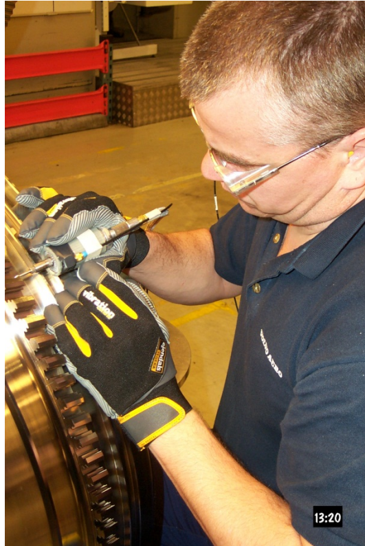
Figure 4: Performing deburring of an aircraft engine component during measurement. The operator is wearing the TEGERA anti-vibration glove.
