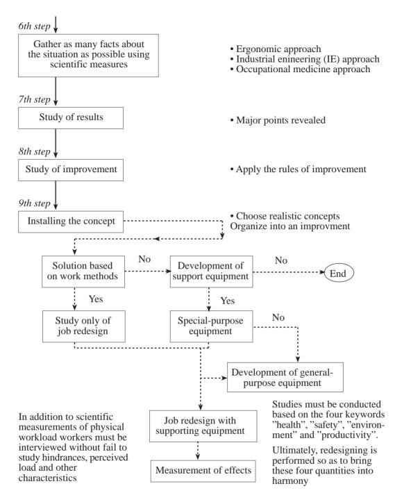
Figure 1. An ergonomic approach to support older workers in assembly line through the development and introduction of support equipment to reduce workloads and enhance productivity.
