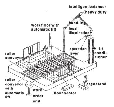
**Figure 2.** Design of multifunctional workstation for an assembly line in a flexible manufacturing system.
