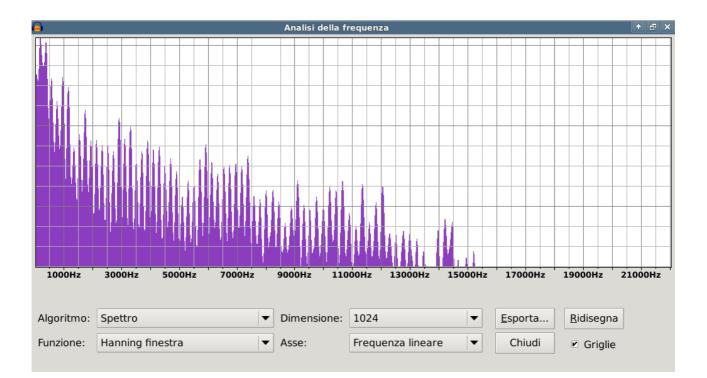
**Cypress** has perhaps the most distinctive spectrum: it has a strong octave, while subsequent overtones decrease rapidly in presence until the obvious leak at around 2000Hz. After this point two other strong areas around 3000-3300Hz and 6000-6200Hz are visible on the graph.
