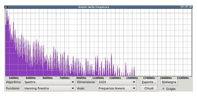
**Spruce** produced the smoothest graph and, especially in the lowest range, also the boldest one. This means that the low range of the frequency spectrum is particularly loud. In fact it shows a very strong octave and the following overtones are remarkably present until the nineteenth.
