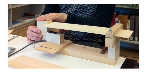
Clamping the free end of the board before performing the vibrations' decay test.
