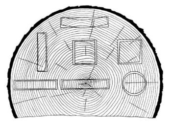
Speaking of instrument building and soundboards in particular, this easily explains why quarter-sawn wood is so sought after:<sup>9</sup> considering a typical ca. 75 cm wide, quarter sawn,
