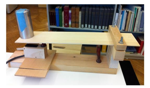
Measuring the sample's bending at the given position.
