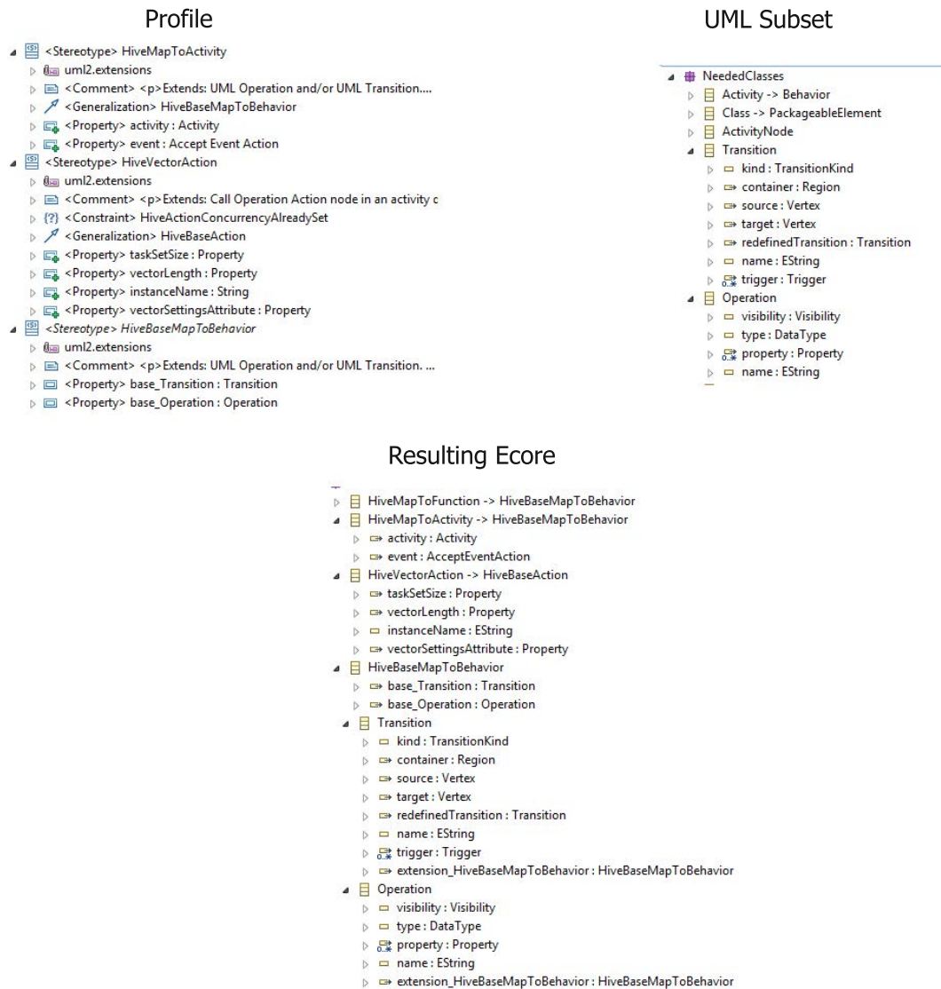
FIGURE 5.7: Part of the Hive Behavior Profile, its UML subset and the resulting Ecore after transformation.
