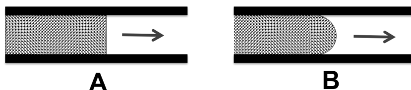
Figure 12. Characteristic flow profiles in CE and HPLC. A. Plug flow profile in CE. B. Parabolic flow profile in HPLC.
