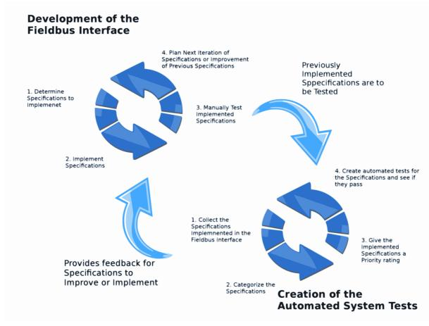
Illustration 2: Automated System Tests Influencing Development of the Fieldbus Interface
