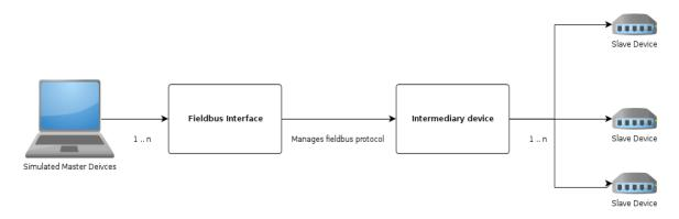
Illustration 1: Fieldbus Interface Integrated in a Test System
