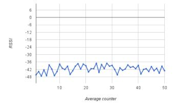
Figure 7. Cave test 1m with adjusted propagation model.
