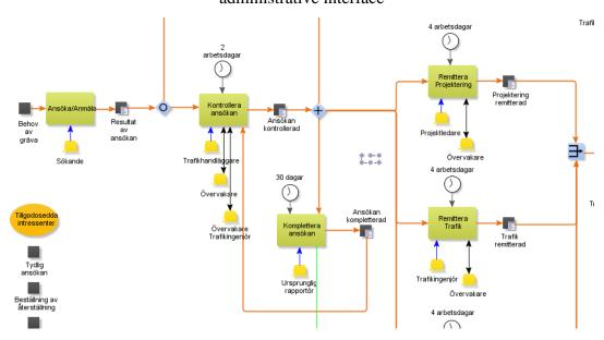
Figure shows the process-map for excavation permits derived during workshops. The figure shows a small part of the process map as to show the map in its entirety would take up to much space.
