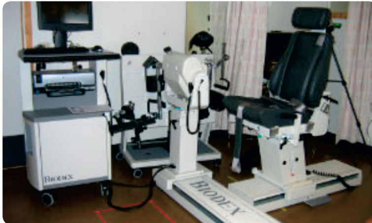
Figure 12 The strength tests were performed using a Biodex machine (Biodex Multi-joint System 4 Pro, Biodex Medical Systems Inc., Shirley, New York). © N. Sernert
