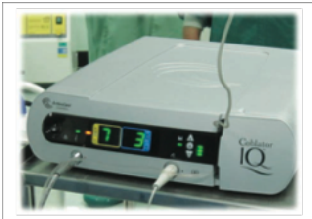
Figure 2. The generator unit to which the plasma ablation debridement probe is attached (Trial et al. Int J Low Extrem Wounds , 2012 Dec;11(4):286-92).
