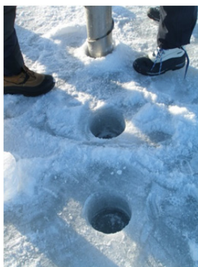
Figure 2. Brine Sampling in Sack holes. Photo: Agneta Fransson
