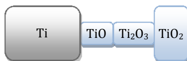
Fig. 7.4. XPS shows presence of \text{Ti}_2\text{O}_3 with Ti in oxidation state +III as an intermediate layer.
