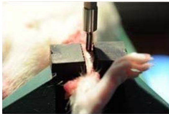
Fig. 12.8. Removal torque (RTQ) is measured using the specially designed abutment for unscrewing the implant during force monitoring.
