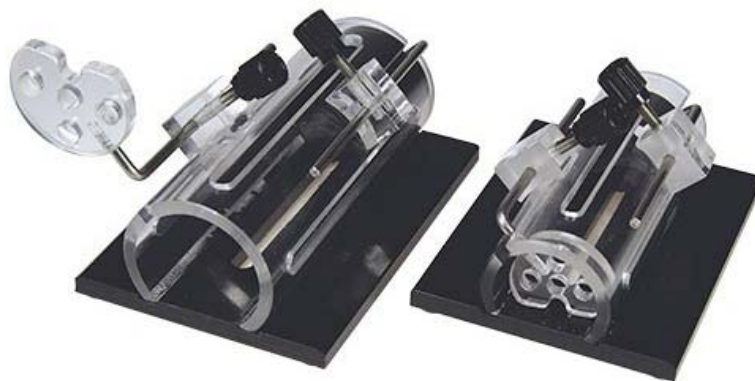
Fig. 12.7. Restrainers for rats of different sizes. To the left model LE5024 for rats between 300-440 grams (AgnTho's AB, Lidingö, Sweden).
