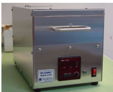
Fig. 12.3. The UVO-chamber emits light at 184.7nm and 253.7nm (Jelight Company Inc., Irvine, USA).
