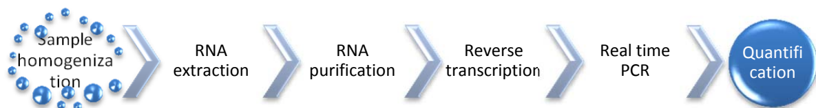
Fig. 12.9. The process of quantitative polymerase chain reaction (qPCR) of implant and peri-implant tissue material.
