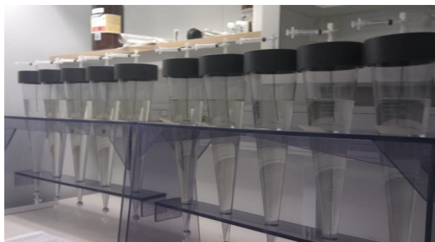
Figure 13. Photography of the experimental setup for the evaluation of sedimentation and aggregation of ENP in MNW. Photo: Julia Hammes
