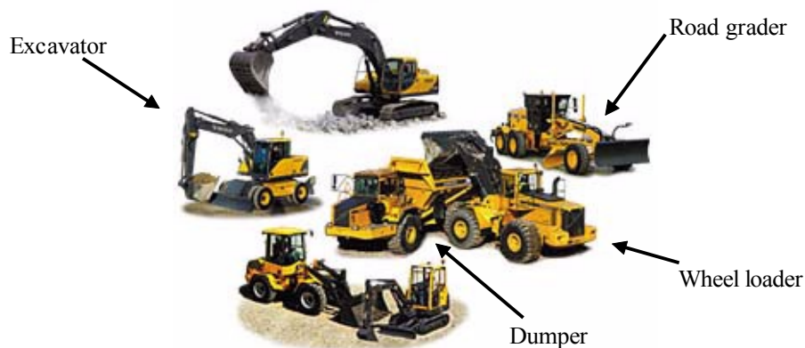
Figure 1:2 Examples of earthmoving equipment.
