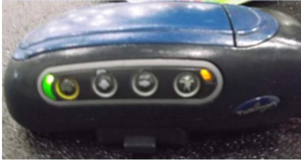
Figure 6 the Talkman T5 hardware showing the four function keys. The picture was taken at the Dagab field study 2013
