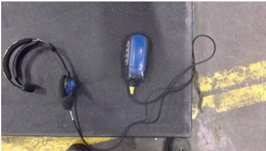
Figure 11 Vocollect ®s Talkman T5 and headset. The picture was taken at the Dagab field study 2013.
