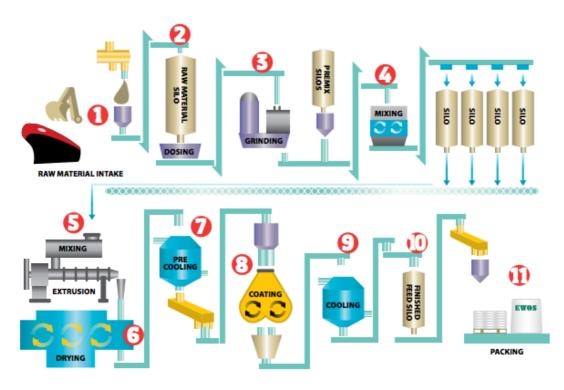
Fig 5.8 Feed Production Process (Ewos 2011)
