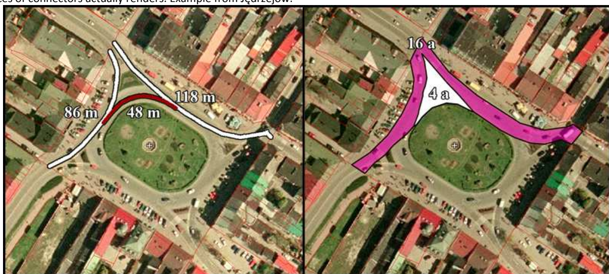
Fig. 6.7. Impact of roundabouts on a market square's cohesion. The left image shows the lengths of two perpendicular roads in a roundabout situation and the length of linking connector. The right image shows how much area in ares (100 ares = 1 hectare) occurrences of connectors actually renders. Example from Jędrzejów.
