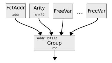
Figure 4.6: Layout of a closure.
