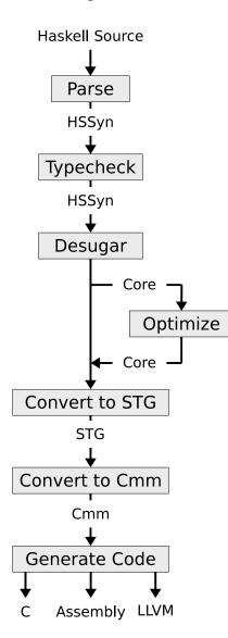
Figure 2.1: The GHC Compilation Pipeline
