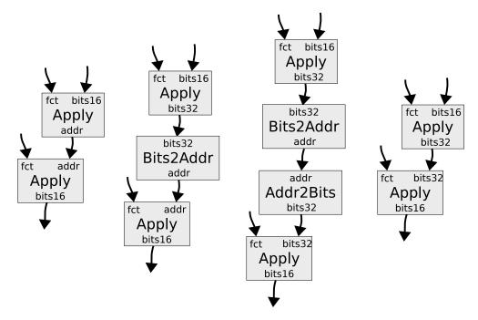
Figure 3.9: The process of type conversion in Jive.
