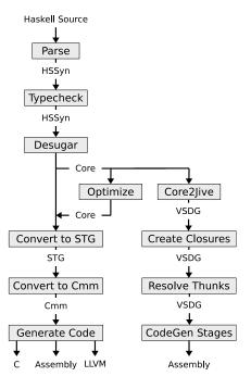
Figure 4.1: The GHC Compilation pipeline with Jive back-end.
