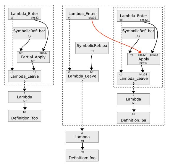
Figure 4.8: The transformation process for partial\_apply nodes.
