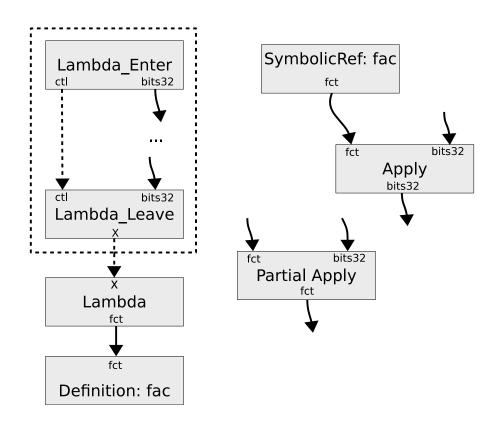
Figure 3.6: Nodes provided for function support in Jive.
