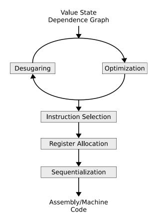
Figure 3.5: The Jive compilation process.
