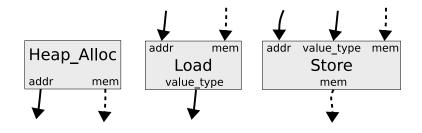
Figure 3.7: Nodes provided for the support of memory operations.
