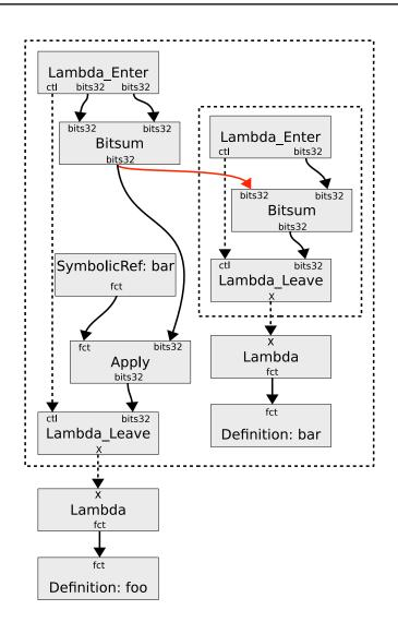
Figure 4.7: Free variables in the Value State Dependence Graph.
