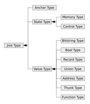
Figure 3.4: The inheritance hierarchy of the supported types in Jive.
