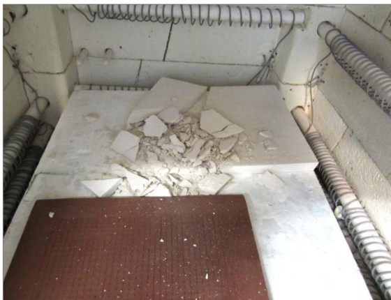
(fig. 18) Exploding during bisque firing
