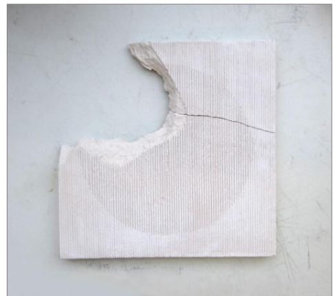
(fig. 18) Exploding during bisque firing
