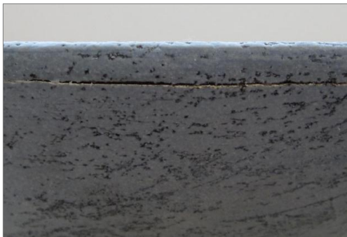
(fig. 20) Cracking after glaze firing
