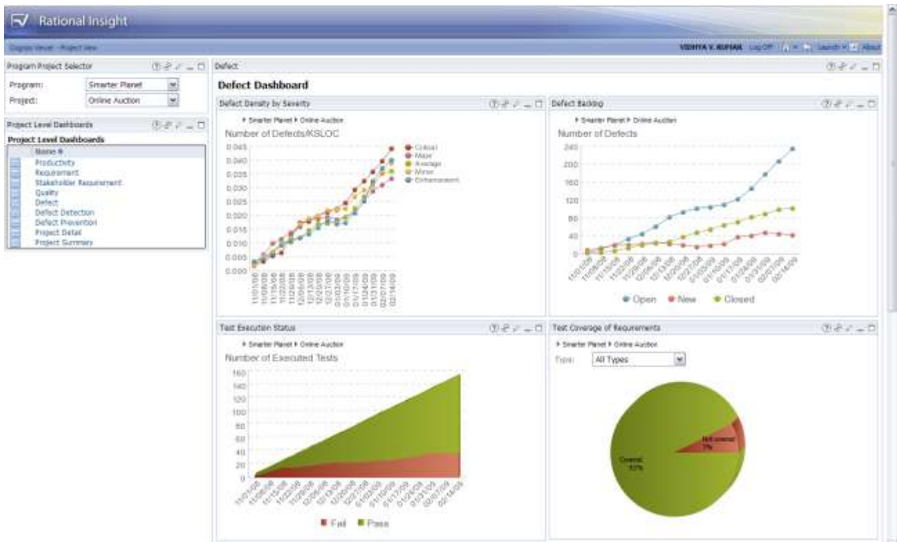
Figure 2 - Rational Insight Dashboard – an example showing defect density, defect backlog, and test execution status
