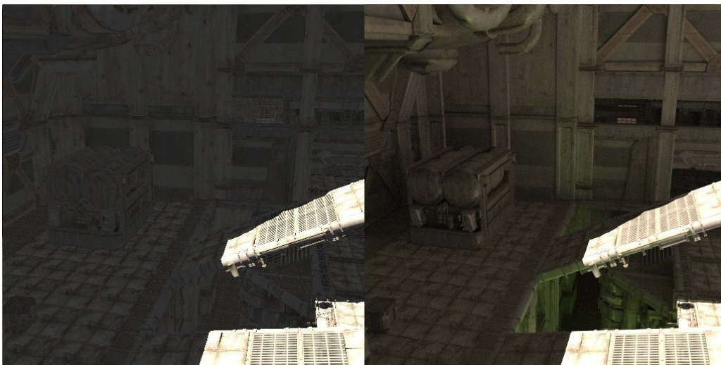
Figure 1: The left image is rendered without global illumination. While the right one is rendered using global illumination with max 4 light bounces. The game level comes from Epic Games, Inc..
