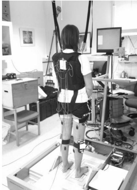
Figure 22 - Force-platform with participant standing facing digital display of CoP and mass-distribution.
