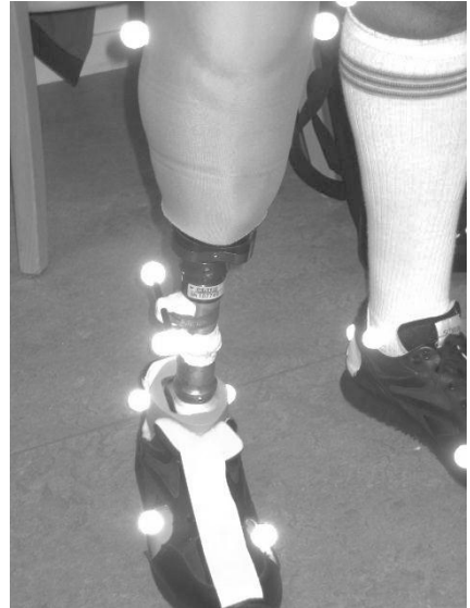
Figure 4 - Reflective marker set-up for a prosthetic limb seen from the anterior direction.
