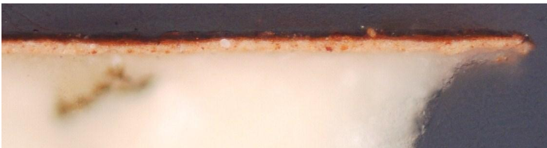
Fig. 49. Cross-section of sample C/Mary Magdalena's red dress (see fig.35-C). The chalk ground is followed by a light red layer composed of white lead, orange and dark red pigment particles. Then a thin red color layer follows. (Photo: Polyxeni Papadopoulou)
