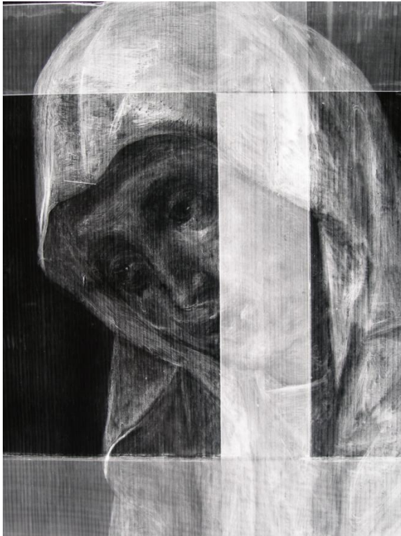
Fig. 57. Detail-Mary. X-radiography. Mary's blue cape has almost equal proportions of lead white as her white veil (bottom left). (SVK, Carin Petterson, Polyxeni Papadopoulou)
