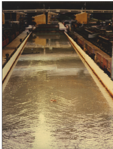
Figure 1.5. A mercury cell in a chloralkali plant. Photo L. Barregård.
