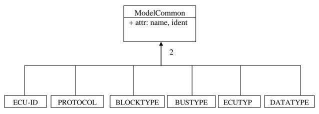
Figure 4.0 – Showing how different classes with same data (name and ident) inherits attributes from the ModelCommon class.
