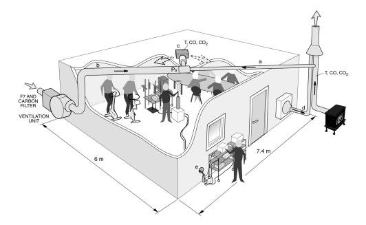
**Figure 3.4.** The chamber (dimensions of 7.4  $m \times 6 m \times 2.9 m$ ) used in **Paper IV**. Partial flow of flue gas (a), flow of filtered indoor air (b), supply of air terminal device (c), ventilation outlet (d), and connection hole for instruments (e).
