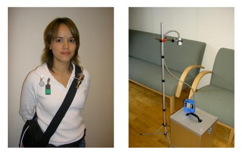
*Figure 3.3 The personal SKC and UMEx samplers (left) and the indoor PAH sampling equipment (right).*
