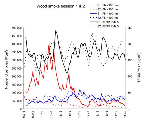
**Figure 4.9.** Particle number concentrations and particle mass  $(PM_{2.5})$ , as measured online using an electric low-pressure impactor (ELPI) and a tapered element oscillating microbalance (TEOM), respectively, during 5.5 h in an exposure chamber with wood smoke
