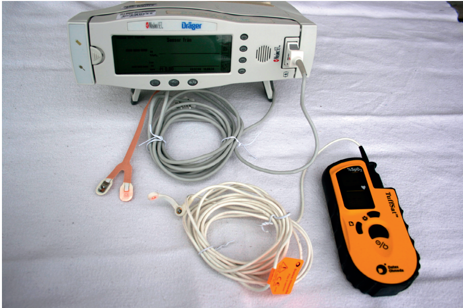
Figure 7. On top the Radical SET with LNOP-Neo sensor and bottom right the TuffSat with Flex II-sensor. The LED are red in the picture. The posey wraps used to attach the sensors and shield them from ambient light are not displayed on this picture.
