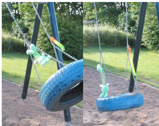
Figure 1: A spiral rabbit and a "slinky" mounted in a swing to demonstrate forces on the rider during various parts of the ride
