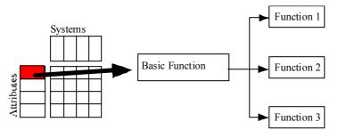
The third step in the process is to determine each systems contribution to the functions, which is performed step by step in the matrix, see figure below.
