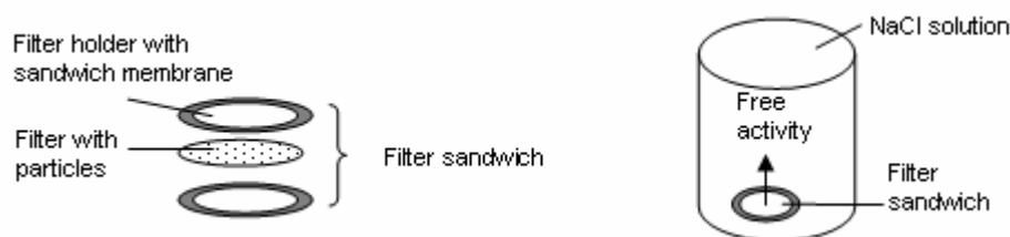
Figure 2. The filter sandwich method. Separation of free activity from particle bound activity in filter with particles.
