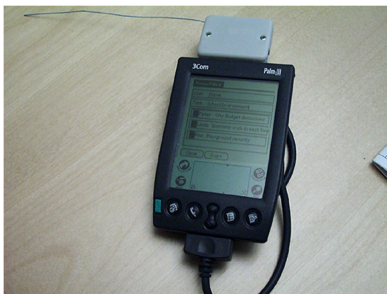
Figure 1. The dynamic to do list runs on a Palm III equipped with a radio transceiver.
