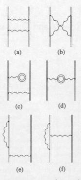
Figure 6.1: Feynman diagrams representing the two-photon contribution to the electron-electron interaction for heliumlike ions. The first row, the "ladder" (a) and the "crossed-photon" (b) diagrams, represent the non-radiative part and the remaining diagrams the two-electron Lamb shift.
