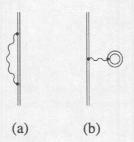
Figure 2.2: First-order radiative corrections, the self-energy (a) and the vacuum polarization (b).
