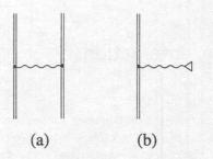
Figure 2.1: The Feynman diagrams for the first-order interactions, the onephoton exchange (a) for two-electron systems, and the one-potential interaction (b) for one-electron systems. The double lines represent electrons propagating in the nuclear electric field, and the wavy line indicates a photon interaction. The triangle represents the interaction with the external potential.
