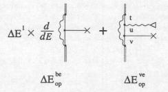
Figure 3.8: Feynman diagrams for the one-potential terms of the binding energy and the vertex correction. The triangle represents the interaction with the external potential and the line with the cross represents the nuclear Coulomb potential.
